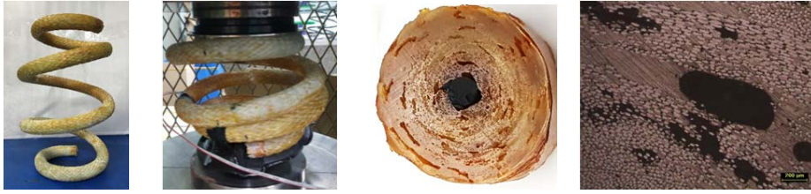
Photo. 1 1 st Coil Spring(Left), fracture during compression test (Middle) and cross-section (Right/Rightmost)
