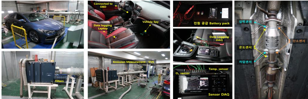
Figure 2. Emission measurement system of dynamometer and location of pressure/temperature sensors
