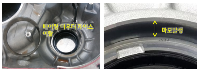
Fig. 1 Outer race looseness due to wear of bearing seat
