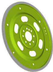
Fig. 1 Shape of Drive Plate for 7-Speed Auto-Transmission
