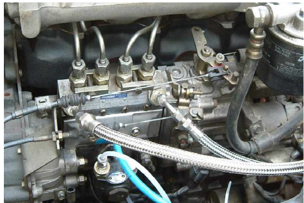
Fig. 3 Modified inline-type injection pump for DME
