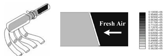
Fig. 6 Pressure drop at the throttle body, viewed through a central cross section.
