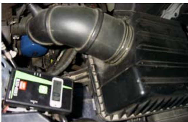
Fig. 12. Electrostatic Measuring at Air Filter
