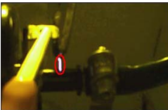
Fig. 8. Electrostatic Discharge at -30°C
