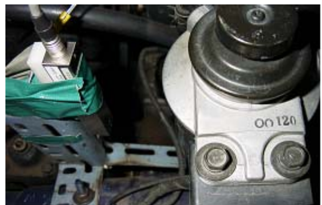
Fig. 10. Electrostatic Measuring at Fuel Filter
