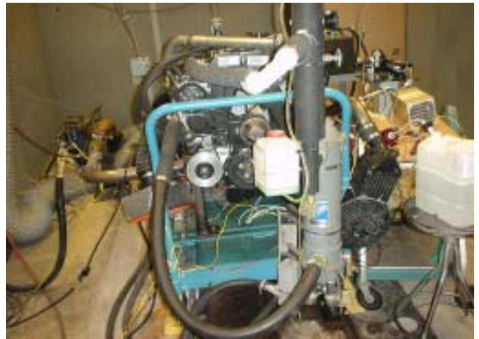
(a) View of engine equipped with a urea-SCR system
