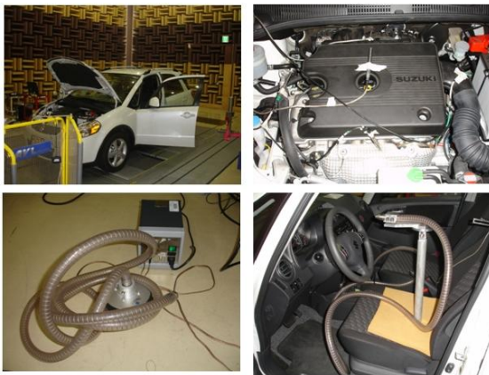
Fig. 1 Vehicle Noise Reduction Test Set-up
