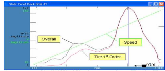
Fig. 1 Steering wheel shimmy at 105KPH
