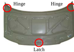
Fig. 5 Original beam type hood
