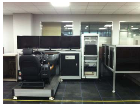
Fig.3 ADAS HILS for Multi ECU Testing
