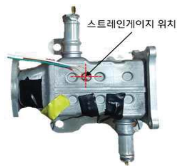
Fig.2 Measurement Point of Strain Gauge in Test
