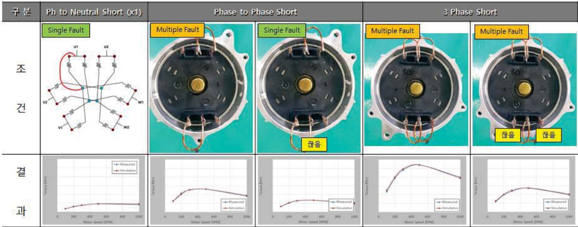
b) Result for Redundant Architecture Motor (Red line : Simulation, Blue line : Test)
