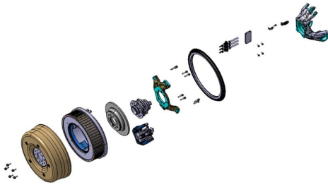
Photo. 1 Direct driven in-wheel system
