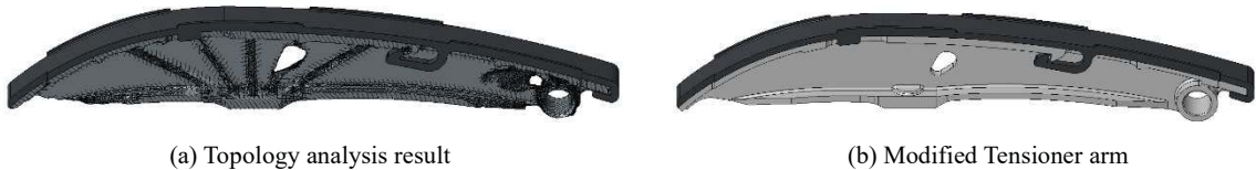
Fig. 2 Tensioner arm bracket modification by Topology analysis
