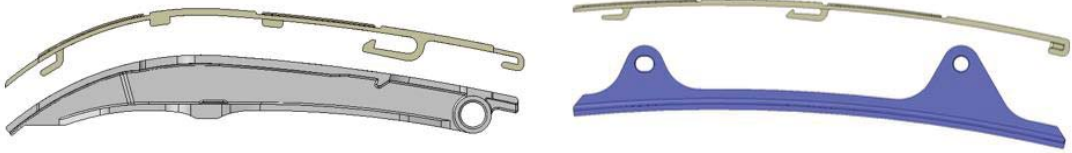
Fig. 2 Configuration of the tensioner arm and chain guide
