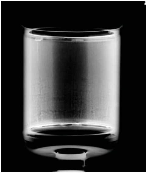
Fig 1. CR-X Image of Hollow Damaged DPF Fig 2. CR-X Image of Melting Damaged DPF
