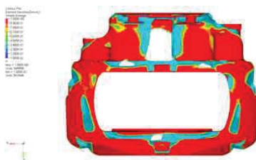
Fig. 1 Topology optimization result of top view
