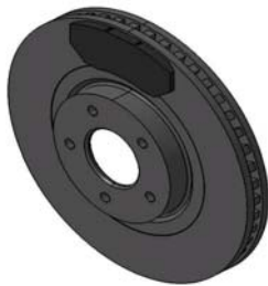
Photo. 1 Disk & Pad reverse engineering CAD file
