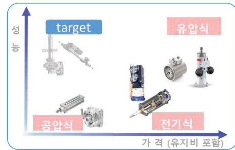
Fig.2 Actuators categorized by kind of power
