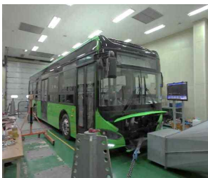
Photo. 1 Electric bus test on the chassis dynamometer
