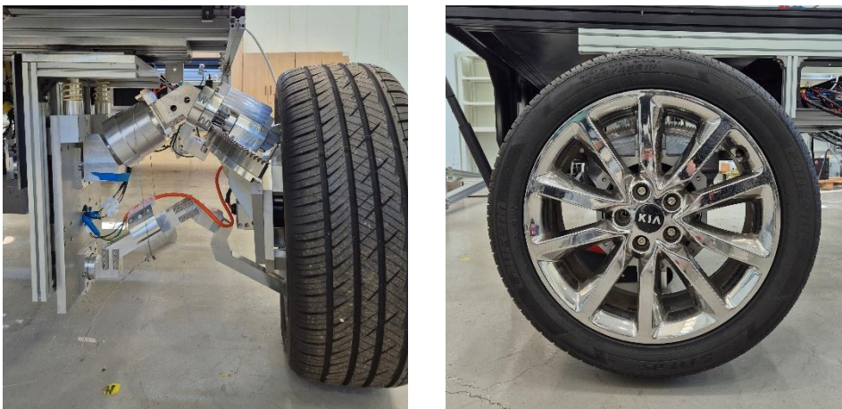
Photo. 2 Experimental set-up of in-wheel motor system
