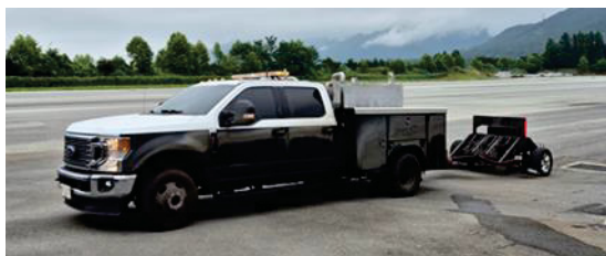
Fig. 1 Wet grip evaluation trailer
