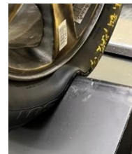
Photo. 3 Deformation of Tire at test
