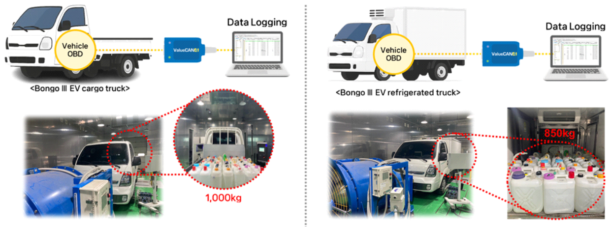
Fig. 1 Diagram of test vehicle and equipment connection
