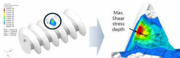
Figure. 1 Maximum shear stress position and stress distribution of worm gear
