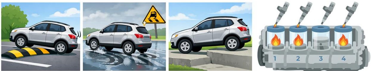
Fig. 1 Common over-torque triggers requiring torque-limiting protection: Tire friction variation, Engine misfiring, Sudden load change
